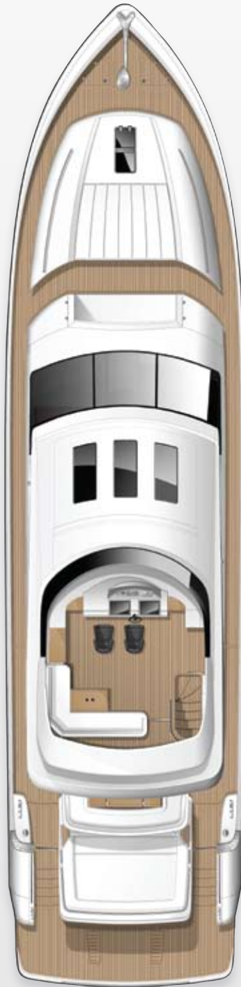
Flying bridge – Dual station control layout
